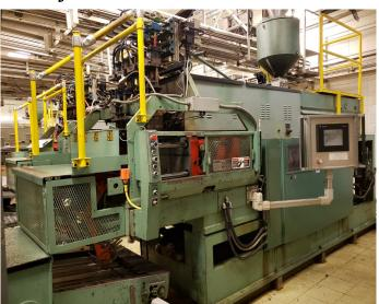
**Rebuilt by UNILOY in 2009/2011 Clamp safety doors Clamp blocking valve** Swing arm retrofit **Auto dump** High flow air **Screw and barrel Trimmer Split Crank Retrofit**
